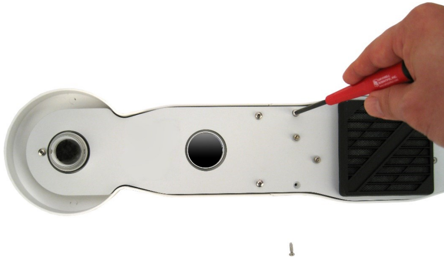
FIGURE C-5. Attaching the solar shield to CNF4 using four flat-head screws
